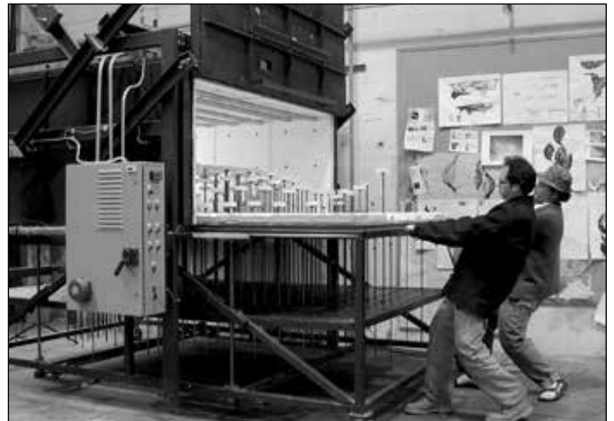
Nikolas Weinstein (l) and Guido Gerlitz (r) rolling out the motorized bed of the full-scale custom kiln (1998).
